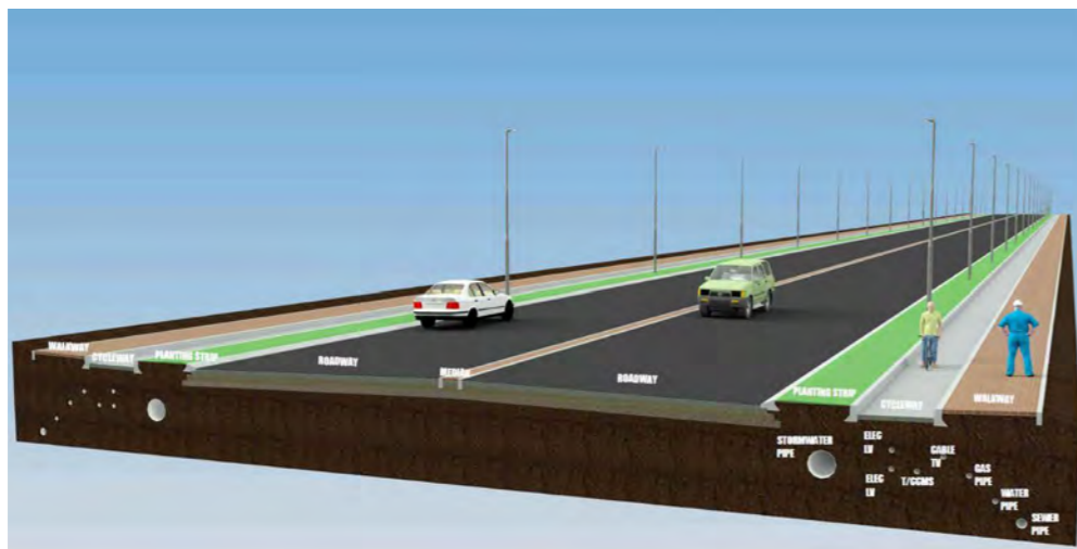
Figure 4.75 Securing of Service Corridors
