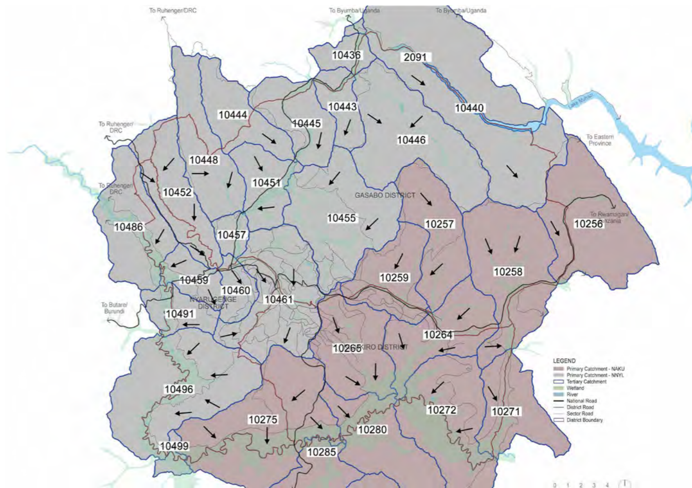
Figure 4.56 Stormwater Catchments Source: RWAF
